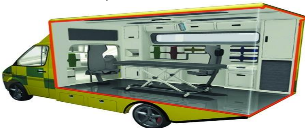
Design features a 'working wall', a patient trolley in the centre of the vehicle and a moulded composite interior
